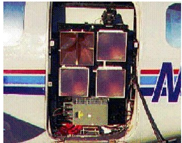
Figure 1. Polarimetric antennas for AT & CT INSAR work, with LN100G INS mounted below, on light aircraft.
